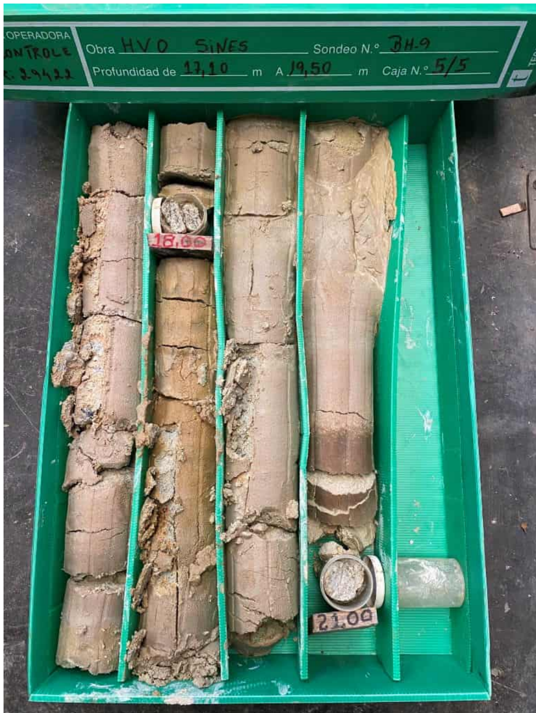
TESTEMONY OF BOREHOLE BH9
