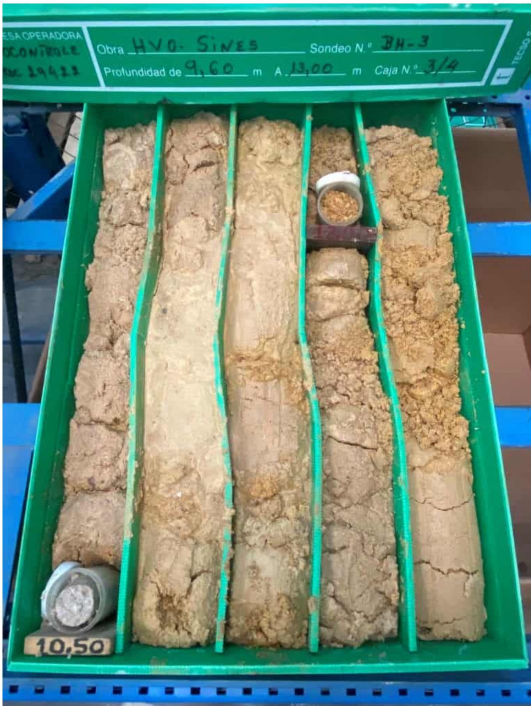
TESTEMONY OF BOREHOLE BH3
