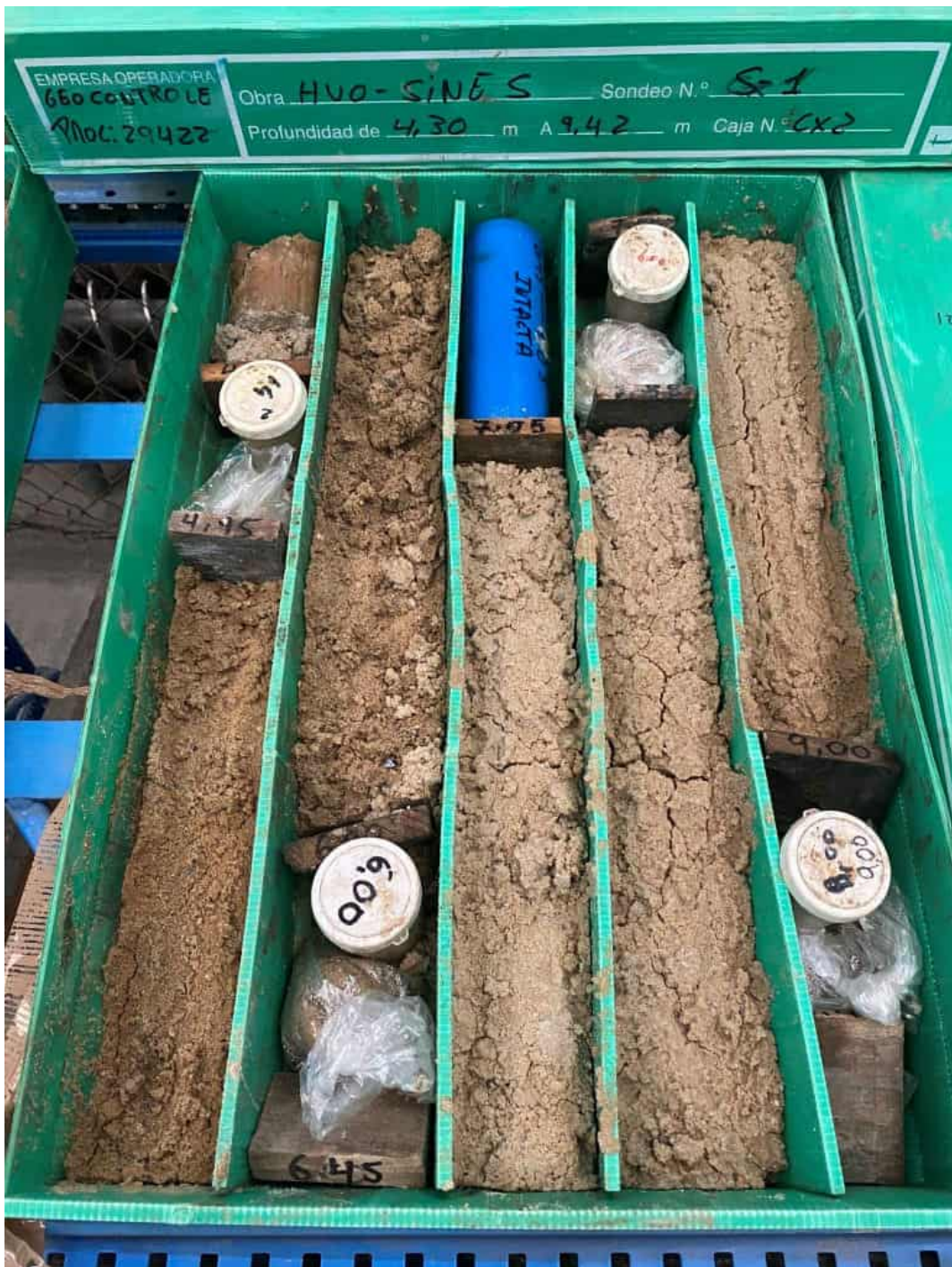
TESTEMONY OF BOREHOLE BH1
