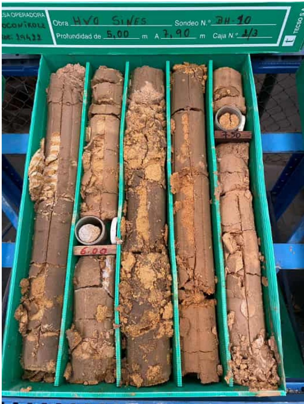
TESTEMONY OF BOREHOLE BH10
