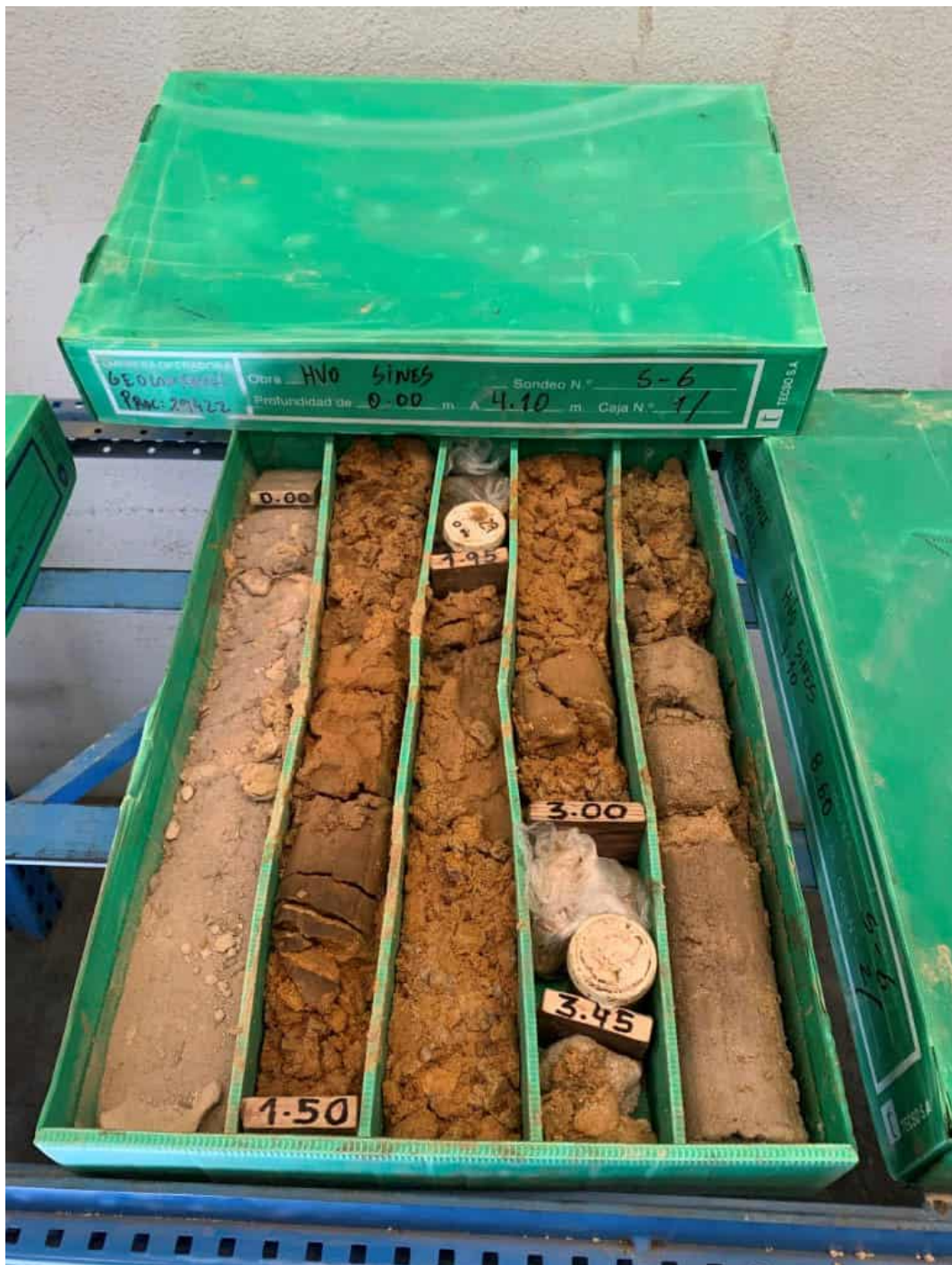
TESTEMONY OF BOREHOLE BH6
