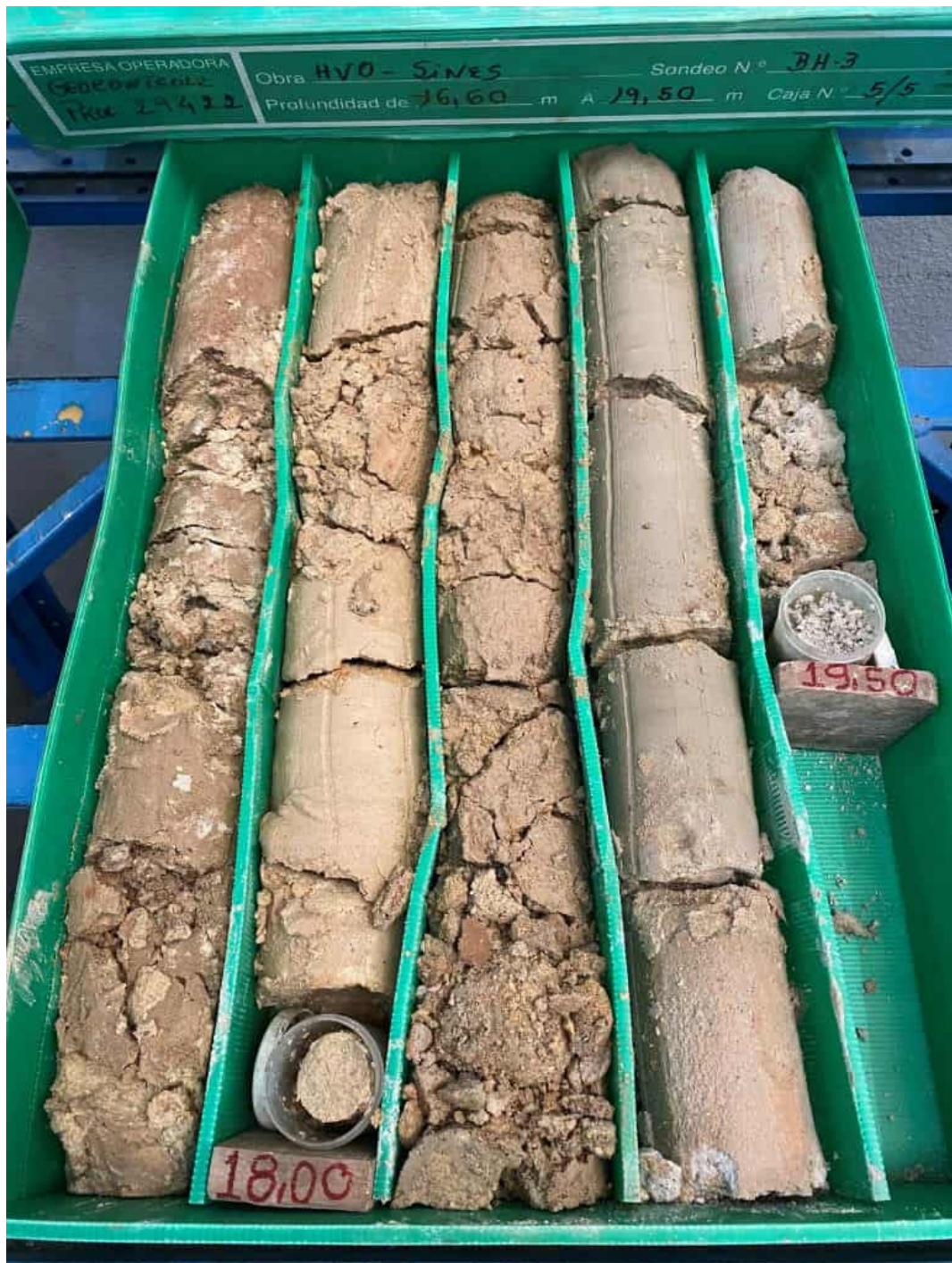
TESTEMONY OF BOREHOLE BH3
