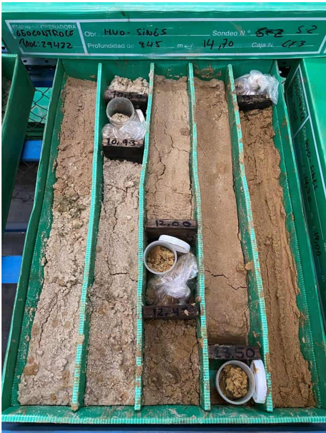
TESTEMONY OF BOREHOLE BH2
