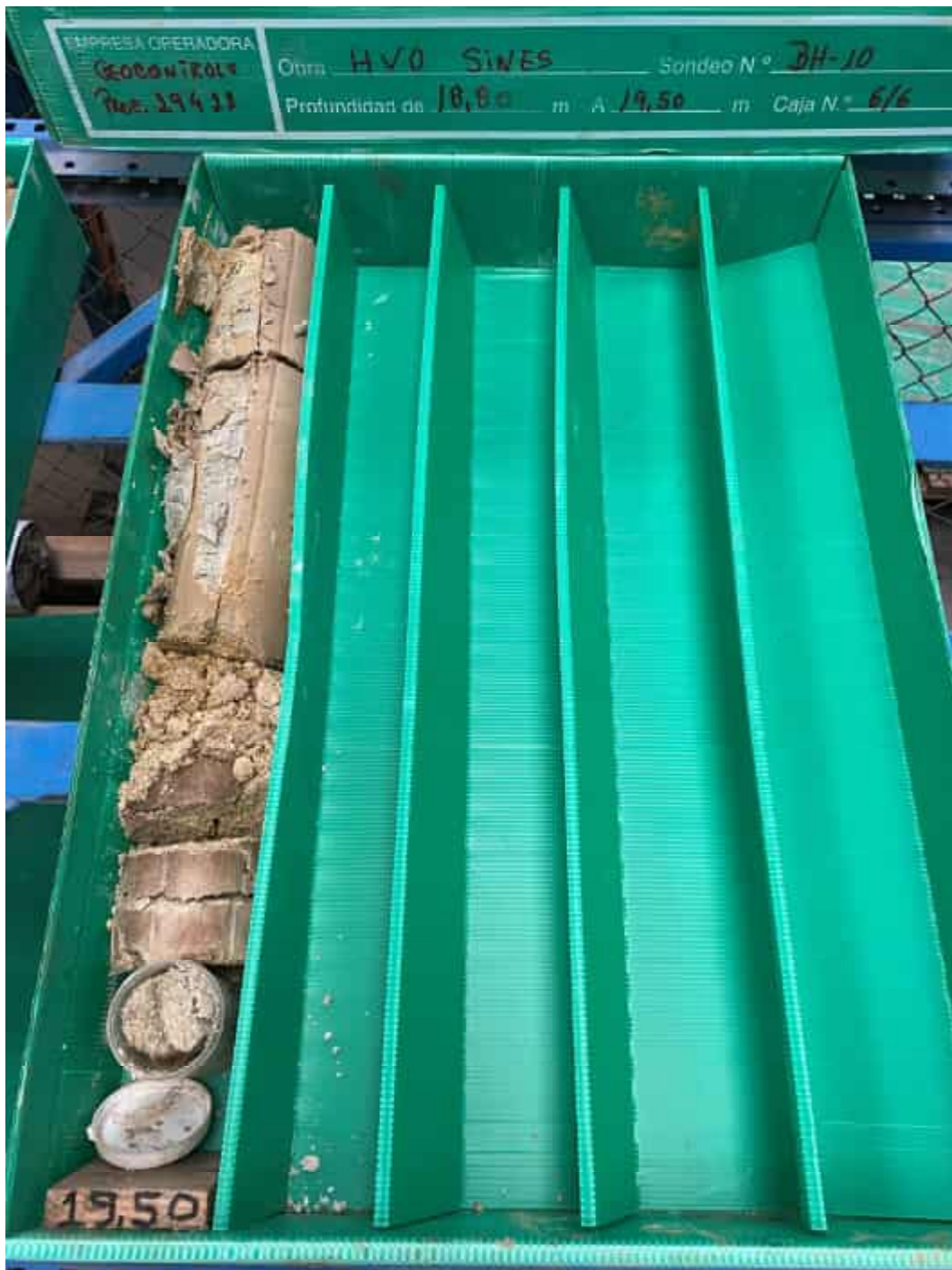
TESTEMONY OF BOREHOLE BH10
