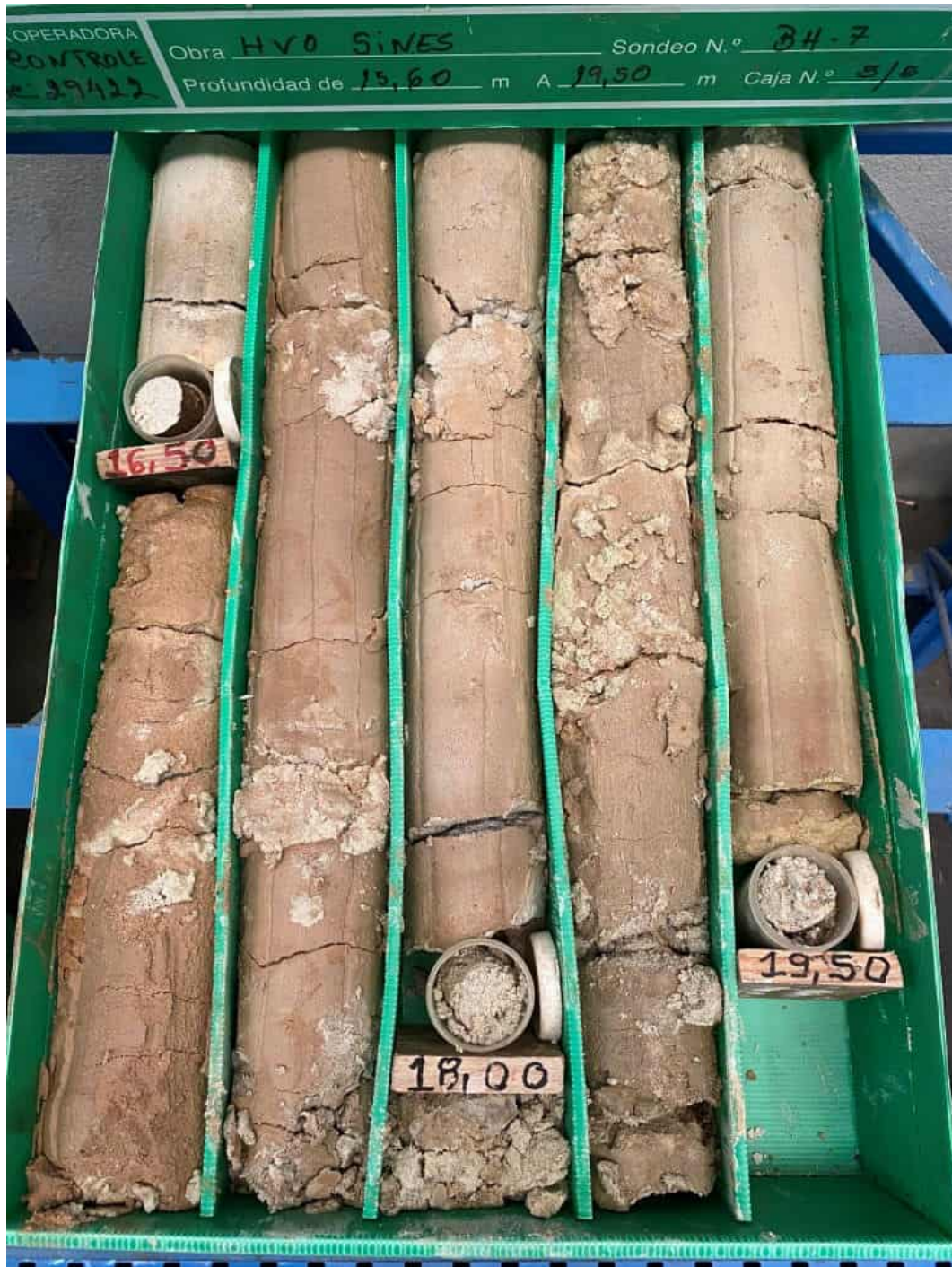
TESTIMONY OF BOREHOLE BH7
