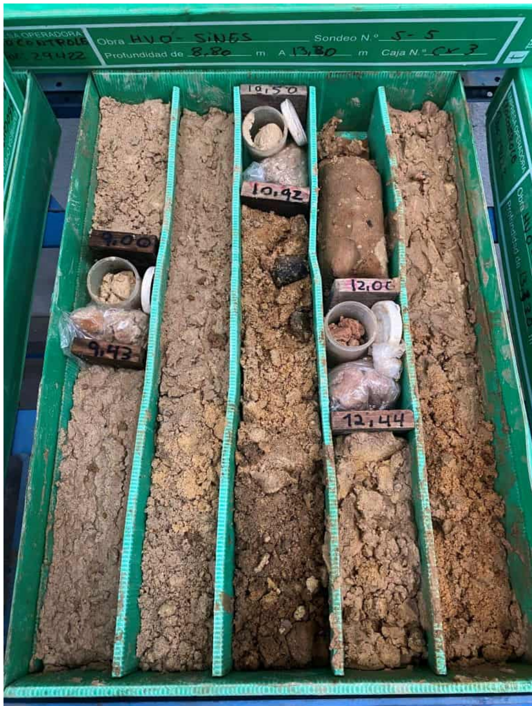
TESTEMONY OF BOREHOLE BH5
