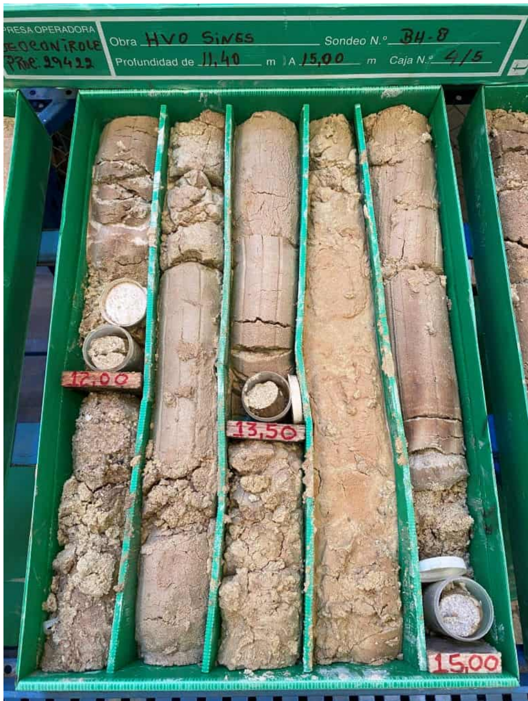
TESTEMONY OF BOREHOLE BH8
