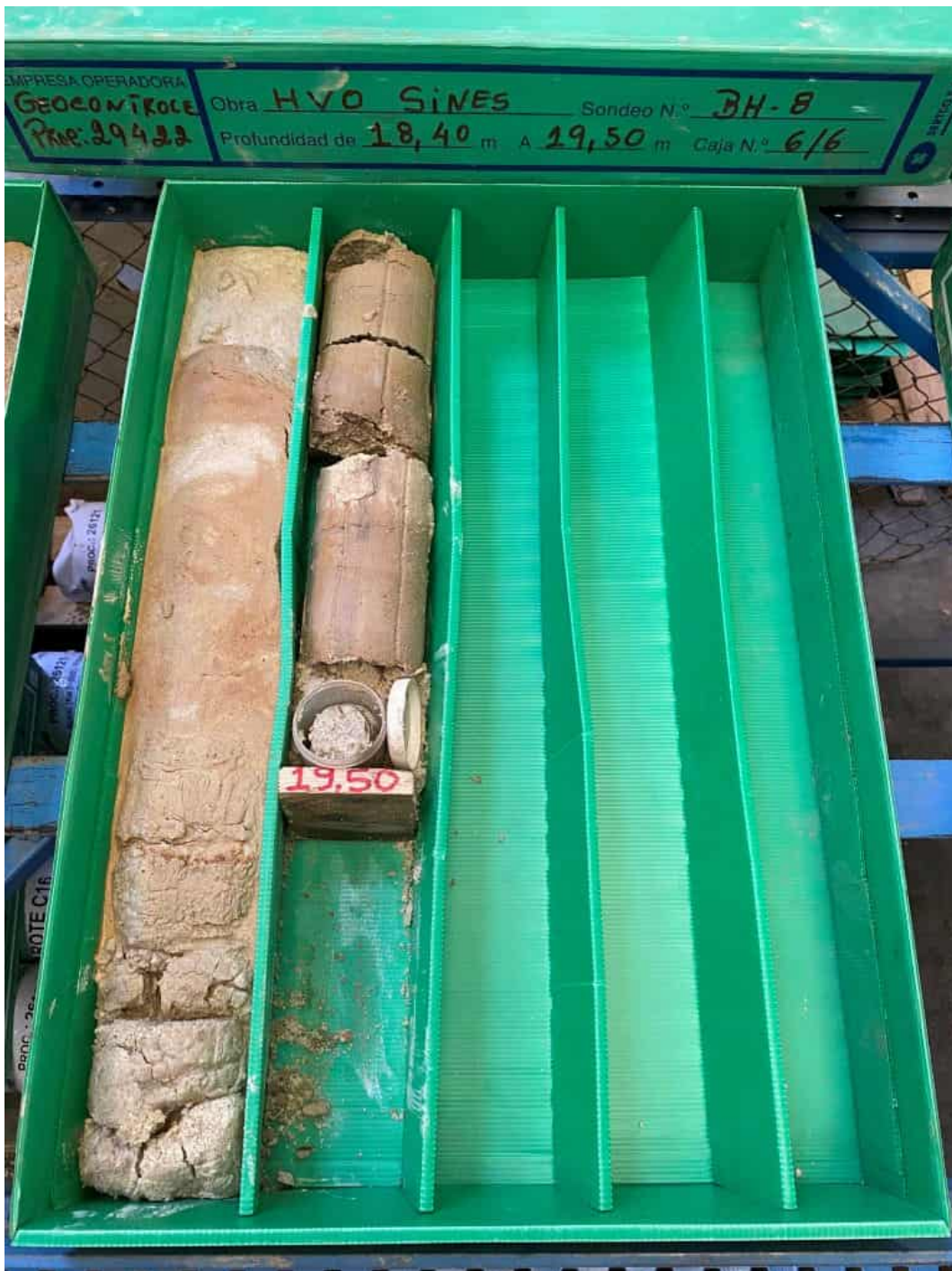
TESTEMONY OF BOREHOLE BH8
