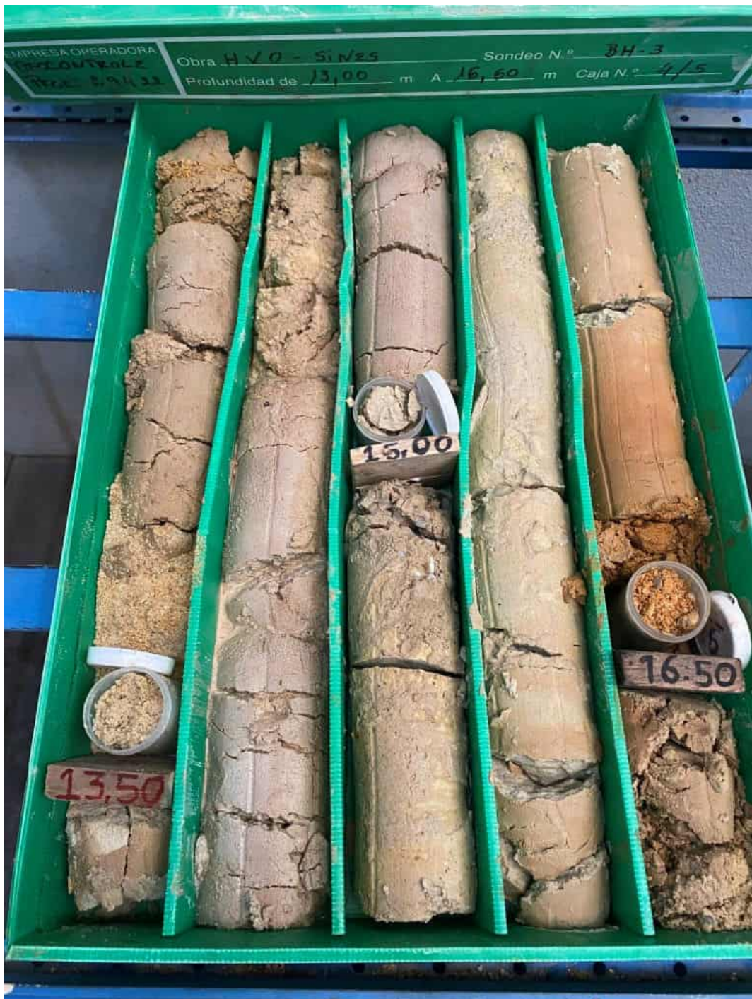
TESTEMONY OF BOREHOLE BH3
