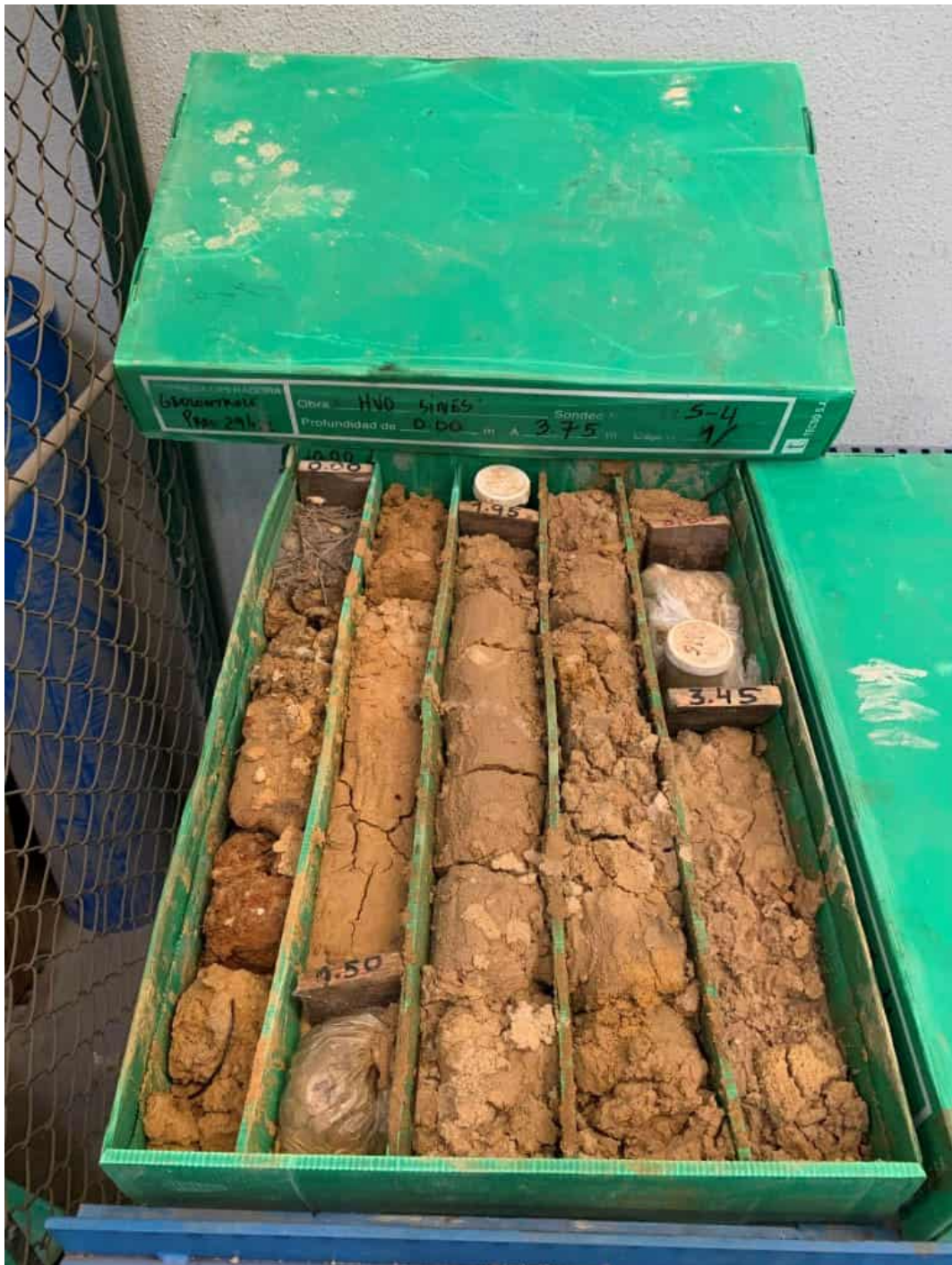
TESTEMONY OF BOREHOLE BH4
