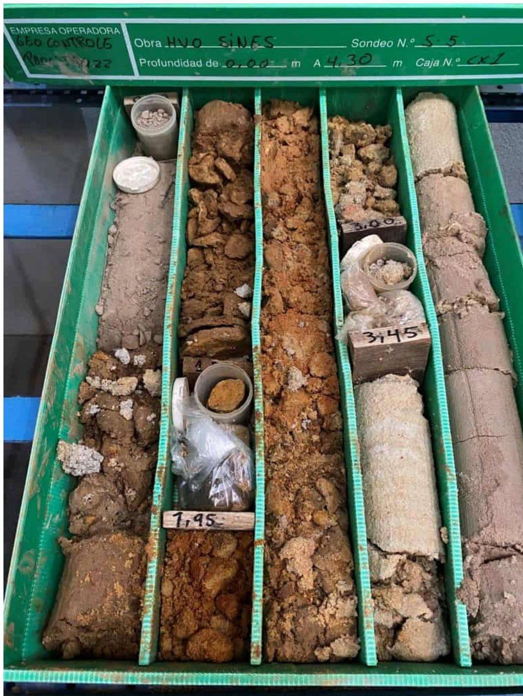
TESTIMONY OF BOREHOLE BH5
