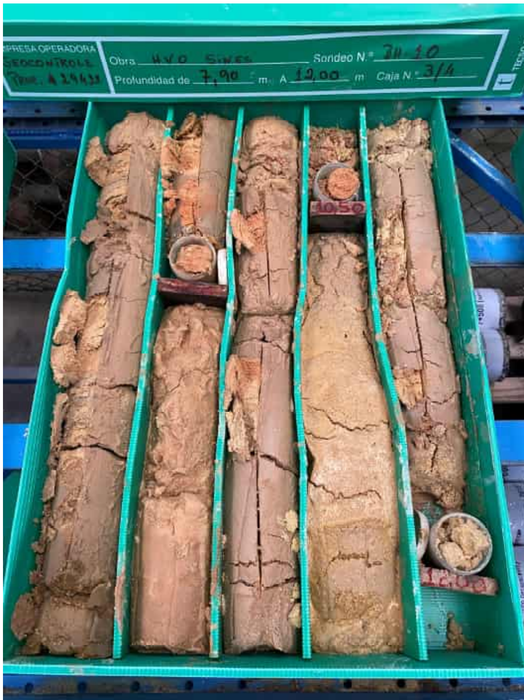
TESTEMONY OF BOREHOLE BH10
