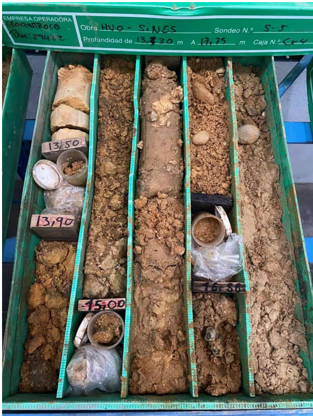
TESTEMONY OF BOREHOLE BH5
