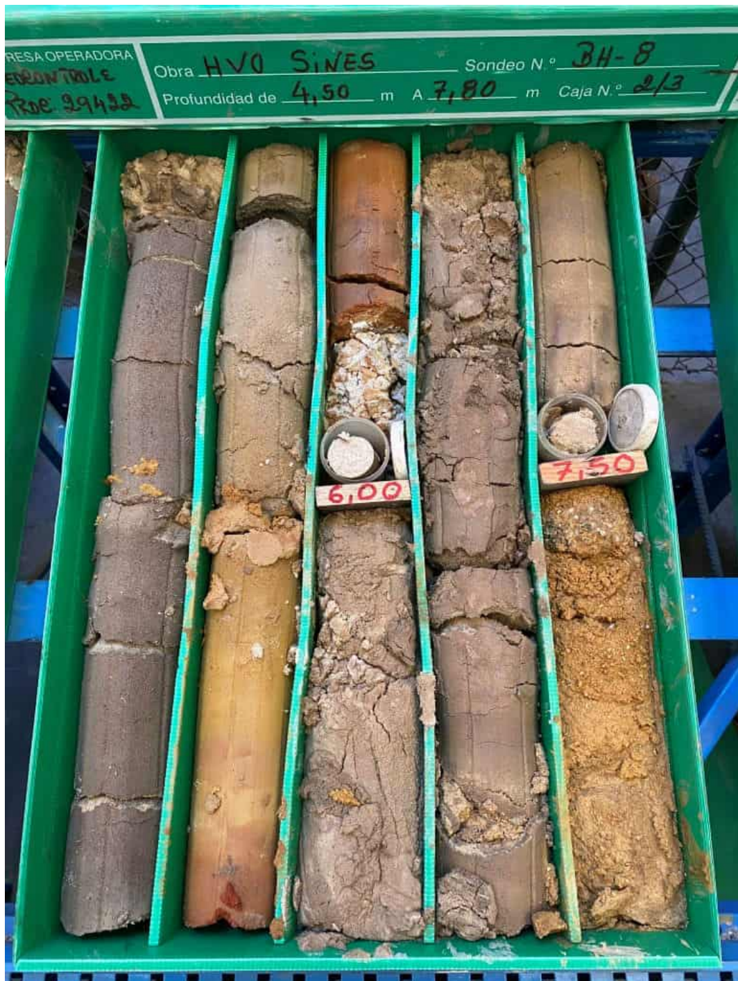
TESTEMONY OF BOREHOLE BH8
