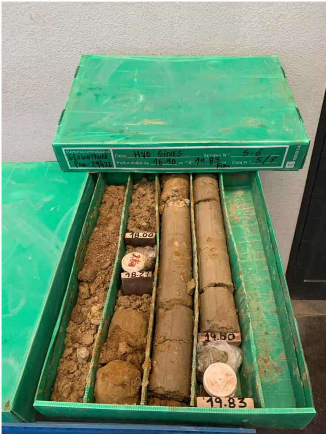
TESTEMONY OF BOREHOLE BH6
