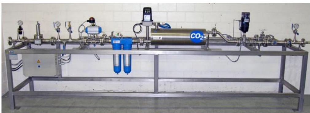
ASCO CO 2 Dosing System (single line)
