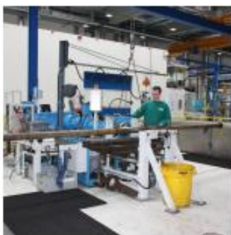
Extruder with stator for oil production
