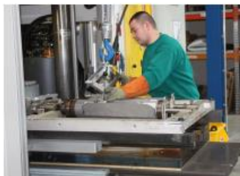
Injection moulding machine for iFD-stators®
