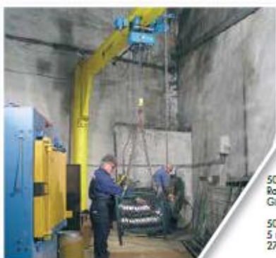
5 t Radio 6 m Giro 360° 5 t 6 m radius 360° slewing
