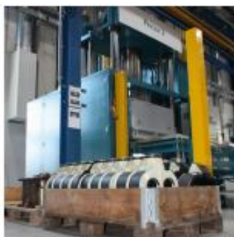
Press with casing liners for TORNADO® T2
