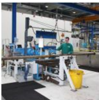
Extruder with stator for oil production
