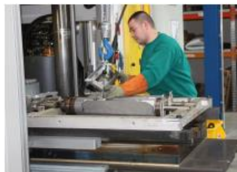
Injection moulding machine for iFD-stators®
