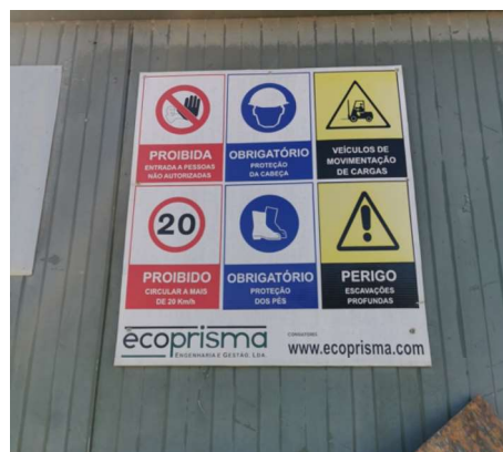
Figure 5: Photographs of the existing signage in the Quarry showing the implementation of the signalling measure of the places that present greater criticality, in the perimeter and inside the quarry.
