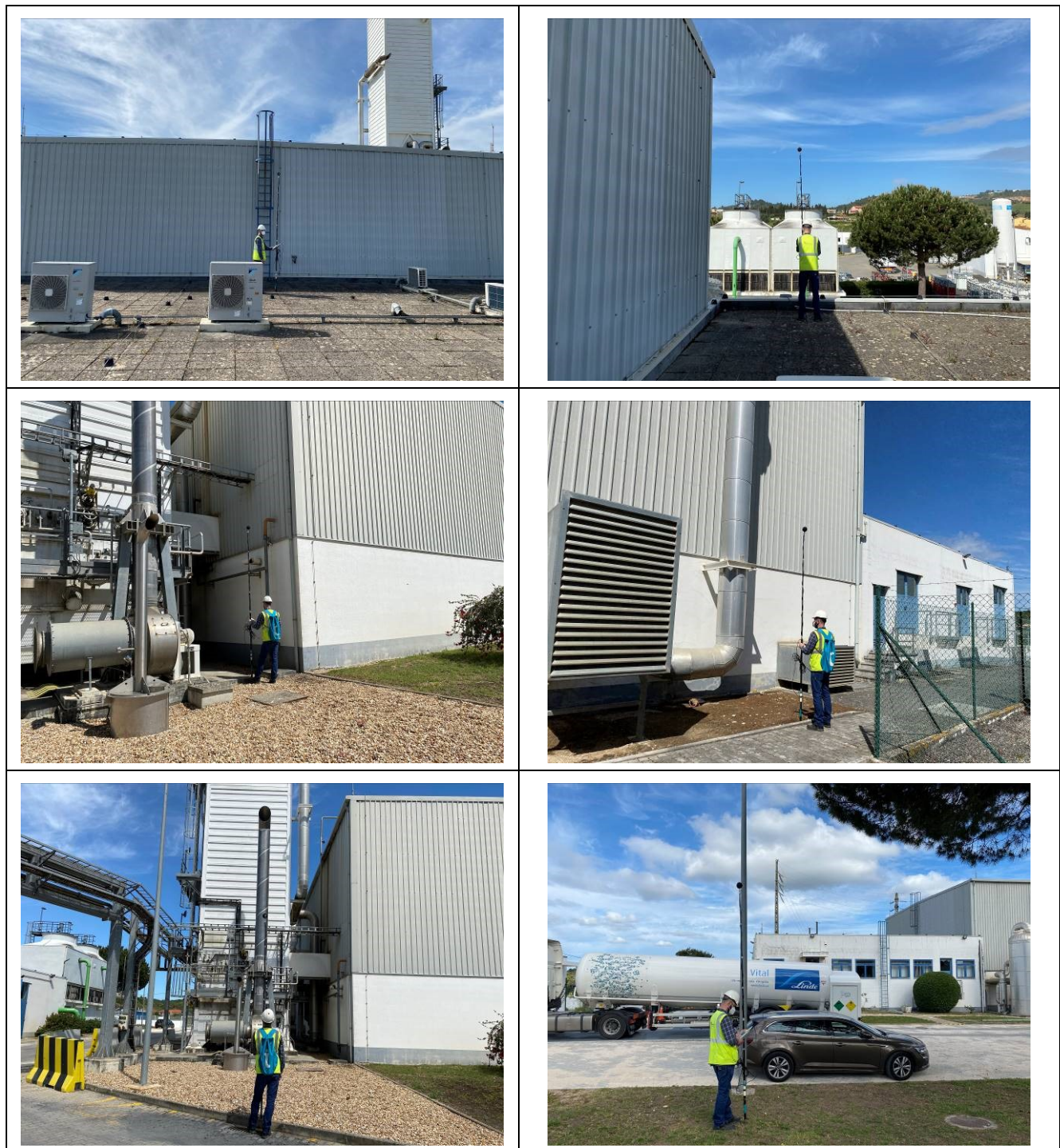
Figure 5-5 – Examples of sound measurements to validate noise sources.
