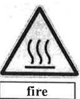
Risks of **BURNS** during the lighting of the firebox and /or the access to the inspection and cleaning doors with firebox lighted or not completely extinguished.
