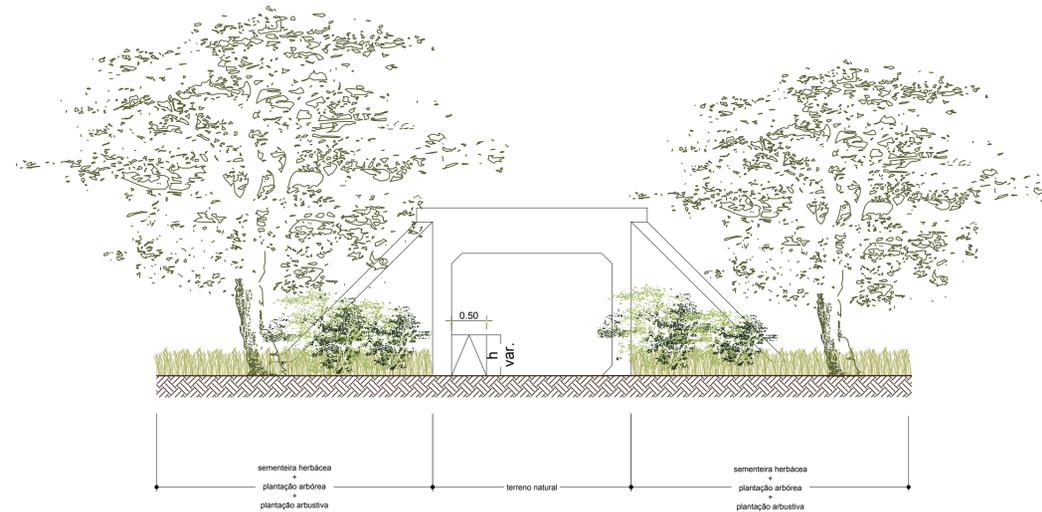
PASSAGEM HIDRÁULICA ADAPTADA PARA A FAUNA COM UM PASSADIÇO LATERAL
